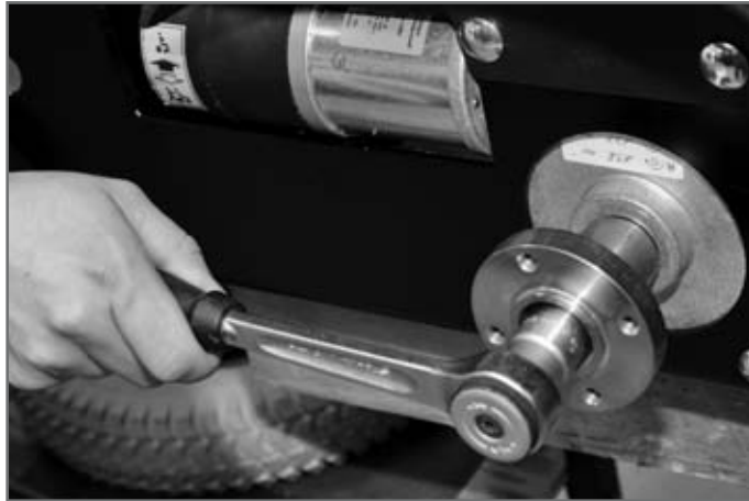
Fig. 22 Loosening the wheel flange screw
