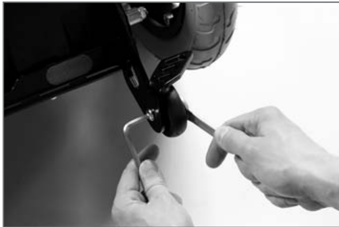
Fig. 26 Replacing the anti-tipper wheel
