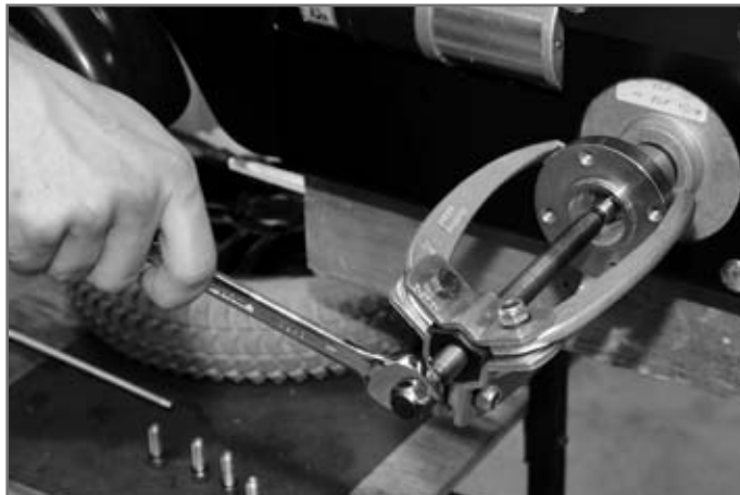
Fig. 22 Loosening the wheel flange screw
