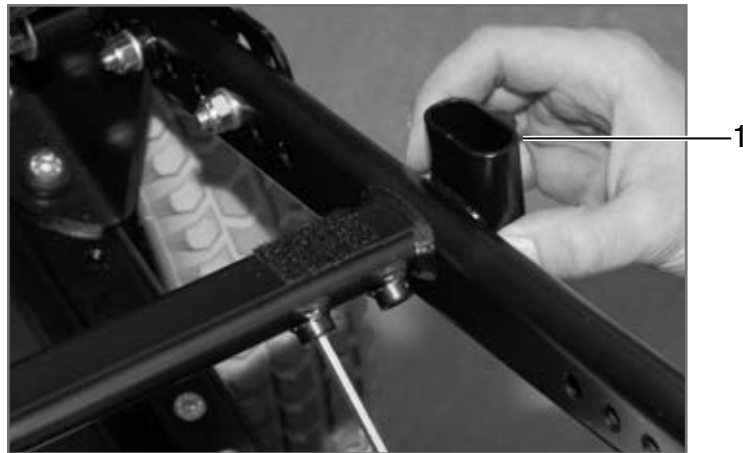
Fig. 36 Replacing the side panel attachment device
