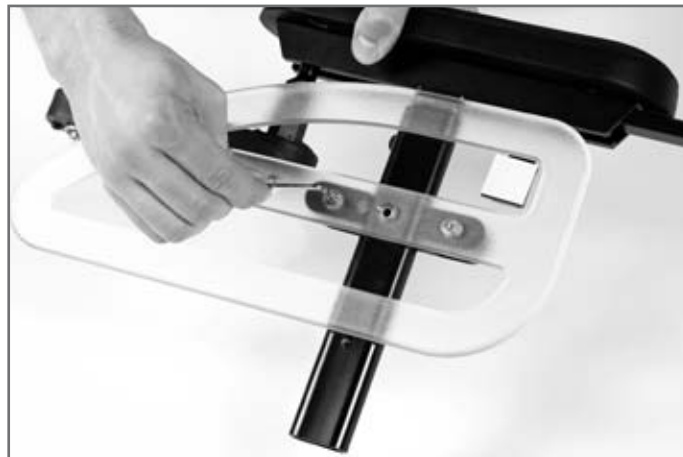
Fig. 13 Replacing the clothing protector
