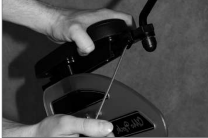
Fig. 44 Retrofitting the rear view mirror
