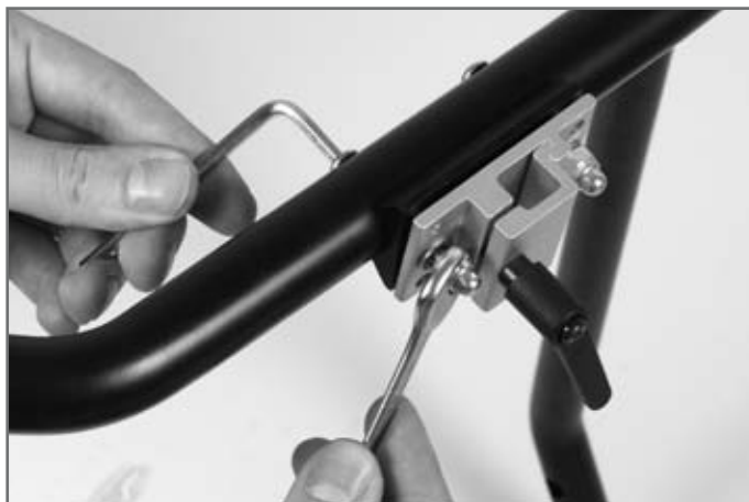
Fig. 45 Installing the headrest installation kit
