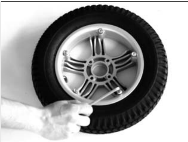
Fig. 20 Removing the casing
