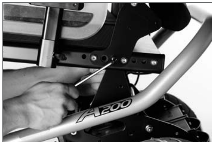
Fig. 34 Standard seat: replacing the seat frame
