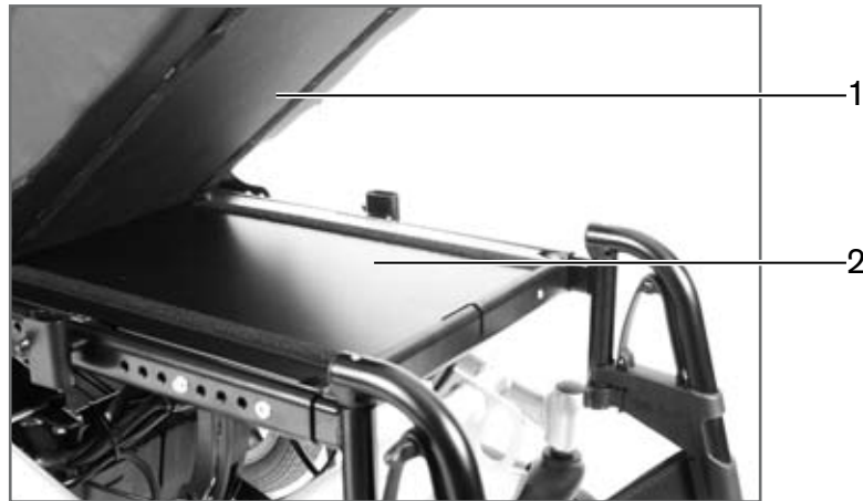
Fig. 33 Replacing the seat plate of the standard seat
