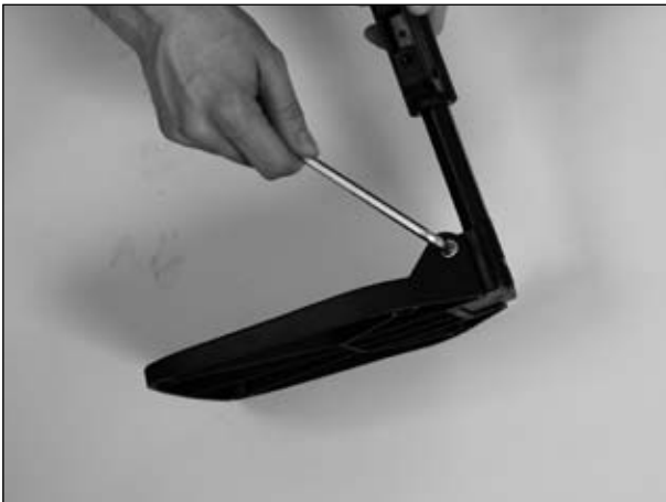
Fig. 19 Replacing the footplate
